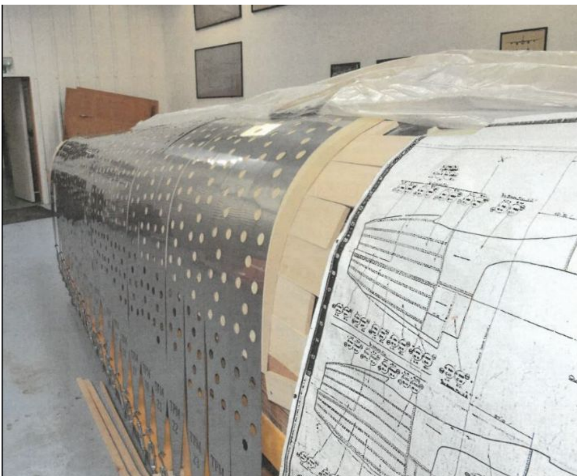
Testing the stainless steel straps for the inner skins.
