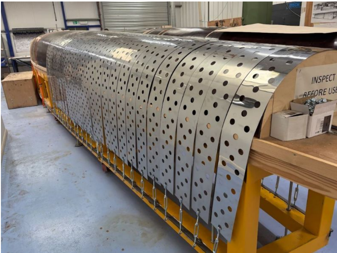
Testing the stainless steel straps for the inner skins.
