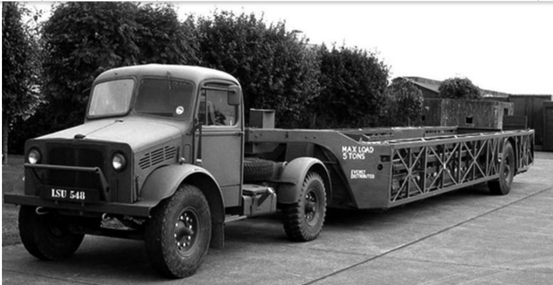
A Queen Mary flat bed transporter, the type used to move Mosquitoes to Ansty for final assembly.
